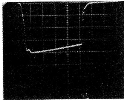
Fig.3 Optimized H + ion beam current. Vertical axis: 5 mA/div. Horizontal axis: 0.1 msec/div.
