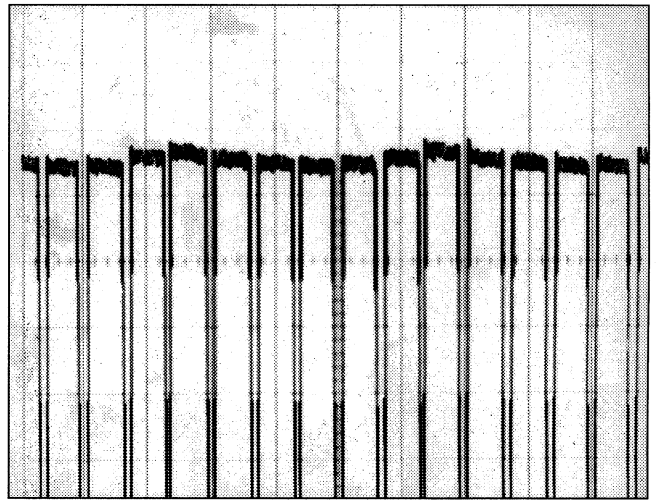
Fig. 4 Powers of RF pulse at exit of accelerating tube 'B11'. The maximum pulse height is 1.8% larger than minimum pulse.
