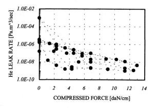
Figure 3: The compression power and a leak rate
