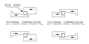
Figure 1: The cross section of a plug and socket
